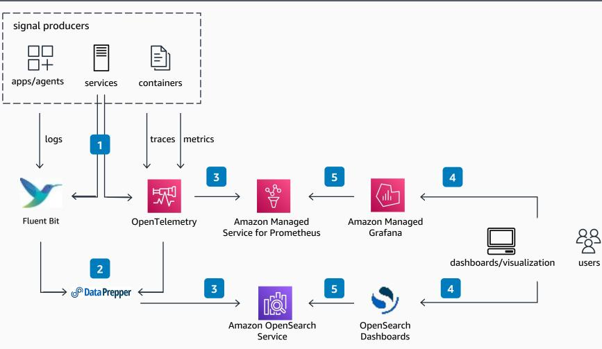
Applications, services, and containers produce three types of signals: logs, metrics, and traces.
