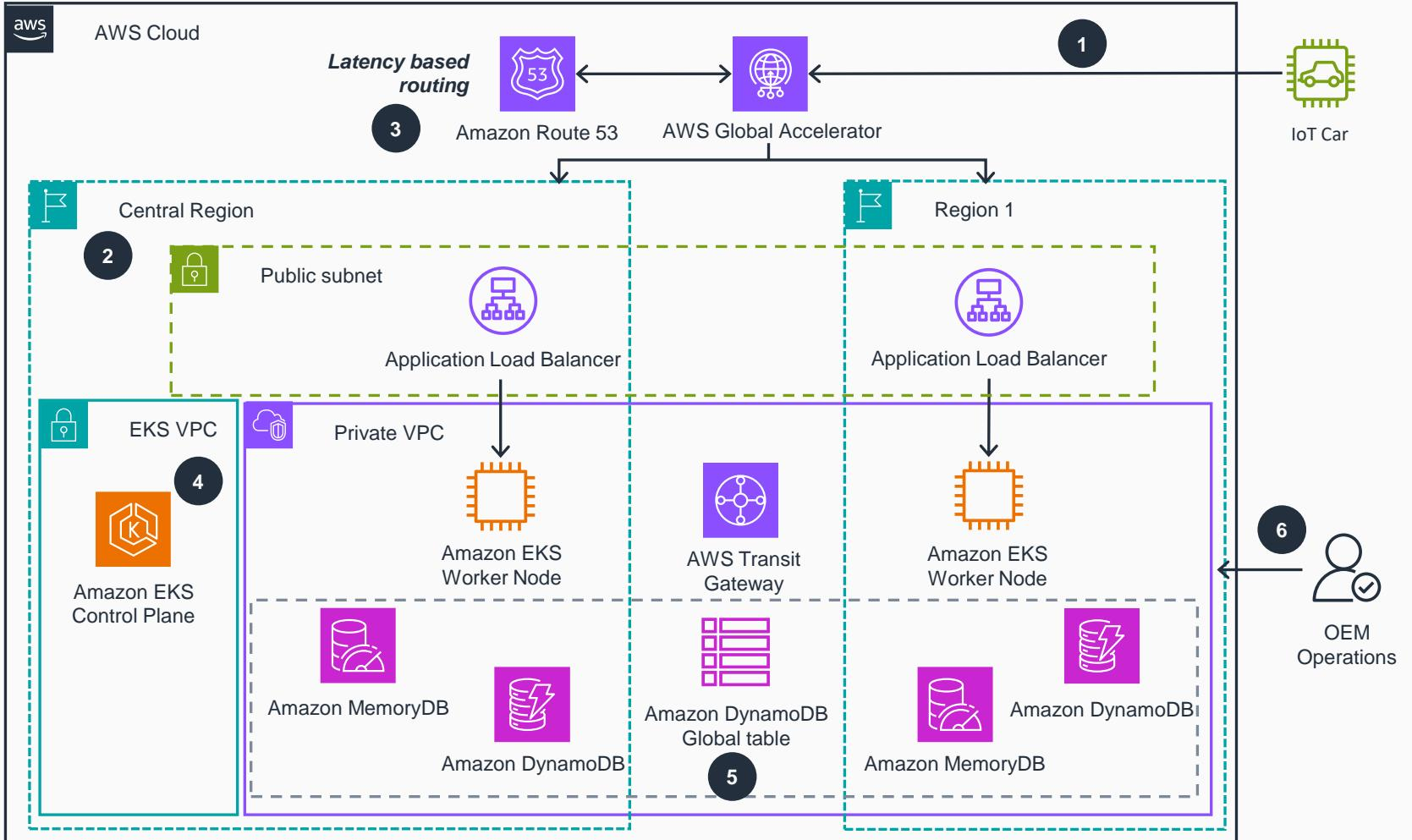
1 Throughout a vehicle's lifecycle, it will periodically check to see if a new configuration exists by calling an **AWS Global Accelerator** endpoint to receive the latest vehicle configuration. To implement a multi-region architecture for Discovery APIs, customers can use **Global Accelerator** instead of building this solution using Amazon CloudFront based on **Amazon Route 53**.
