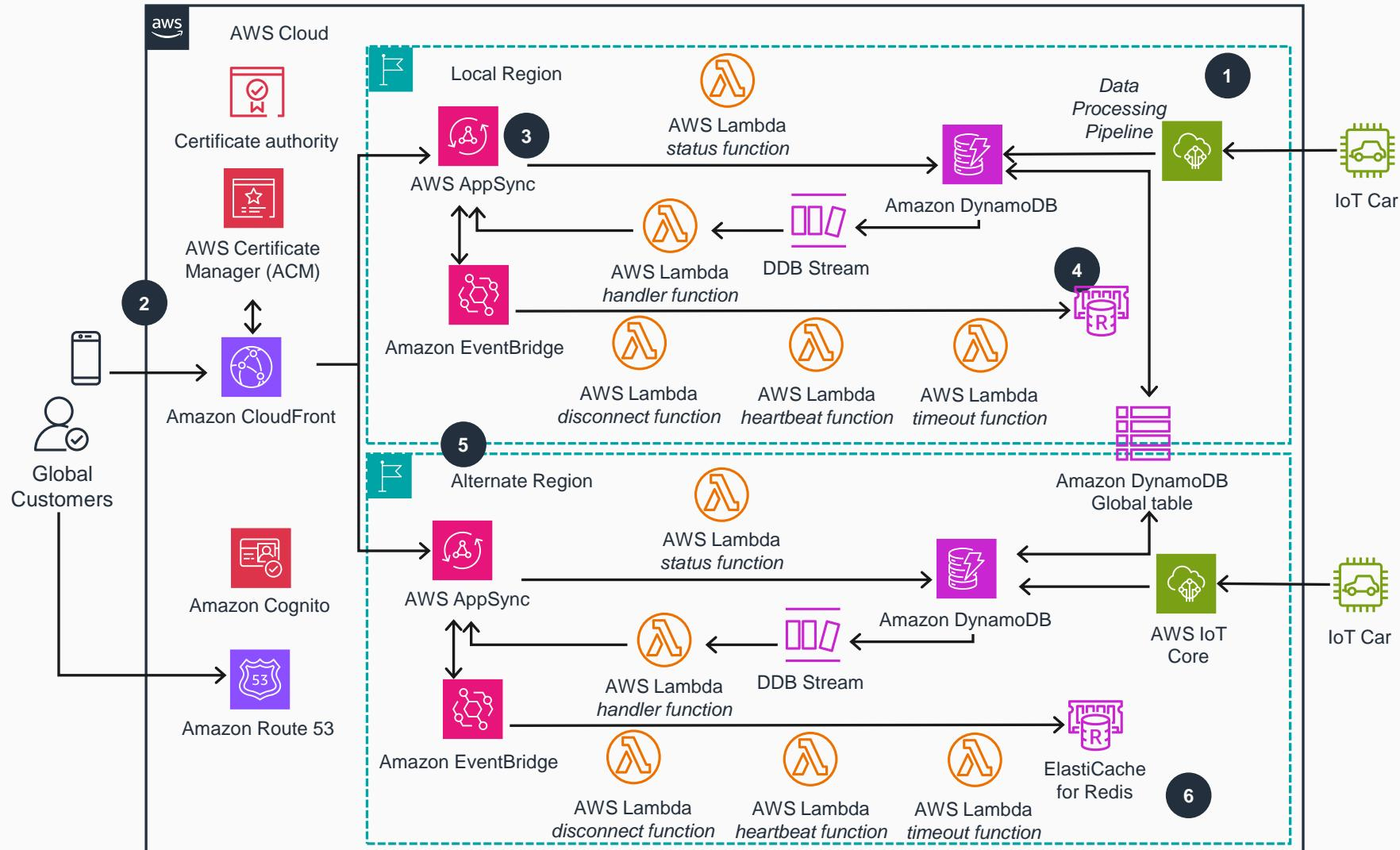
1 Standard data processing pipelines using **AWS IoT Core** as the connectivity layer save the vehicle's Last Known State to **Amazon DynamoDB**. From there **AWS AppSync** provides a GraphQL API to the companion application to deliver the vehicle status to the customer.
