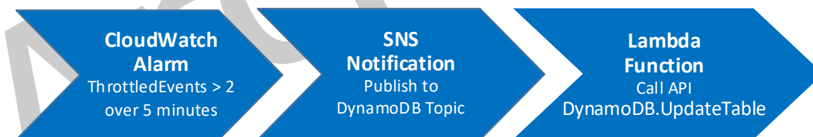
Figure 6: Example of a CloudWatch alarm flow
