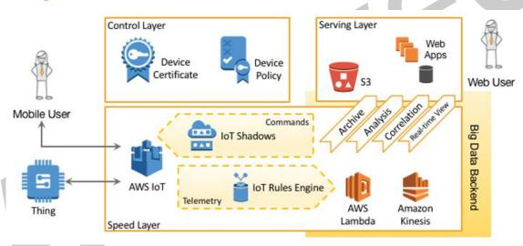
The Pragma Architecture is a single cohesive perspective of how the core tenets of IoT manifest as an IoT solution when using AWS services.
