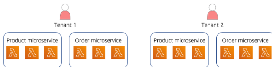
Figure 11 – Lambda Silo Isolation
